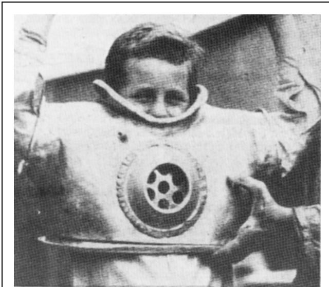
Figure 5. Aubrey Burstall's cuirass jacket respirator, from his original 1938 article. 4 (Reproduced with kind permission of the British Medical Journal.)
